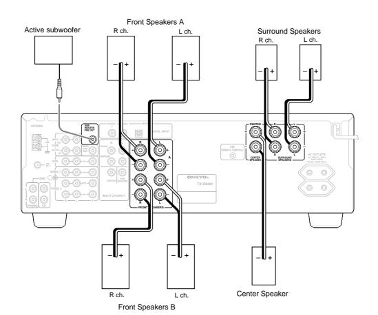
When you use only one speaker or wish to listen to monaural (mono) sound, a single speaker should never be connected in parallel to both the right and left channel terminals simultaneously.
